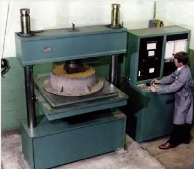
Taking a casting beyond AASHTO M 306 provides ultimate load, maximum deflection, energy absorption and design efficiency.
